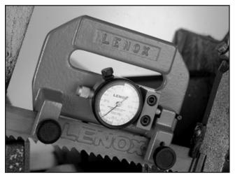
Figure 48. H5408 Blade Tensioning Gauge.
